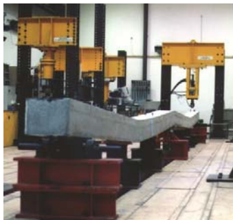
(a) Two-span beam that achieved 99% of full plastic mechanism while exhibiting significant redistribution
