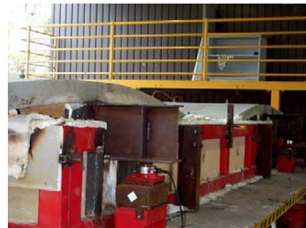
(c) Continuous slab with Ductility Class L mesh subjected to a standard fire – no steel fractured and gross deflections occurred
