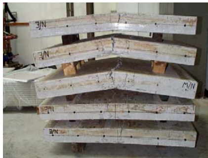
(b) Short slabs incorporating different ductility steels, tested with a central line load until fracture of steel reinforcement occurred
