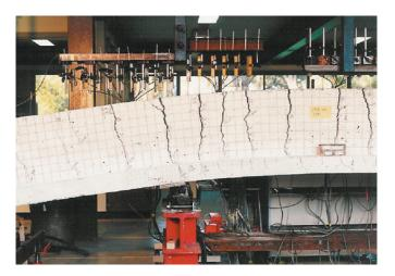
Tests and moment-curvature analysis already confirm that the Class L steel is sufficiently ductile to use simple-plastic rectangular stress block theory to calculate the moment capacity of beam and slab cross-sections.
