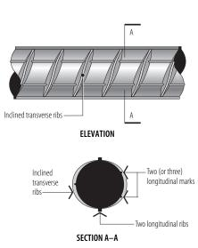
**FIGURE1** General Identification of QST (Straight) 500N Bars
