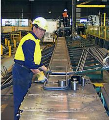
**FIGURE 4** Factory Bending around Pins of Specified Diameters
