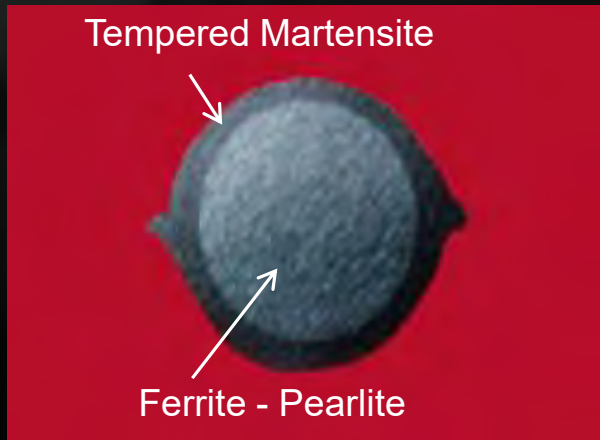
Quenched and self-tempered bar from 1983
