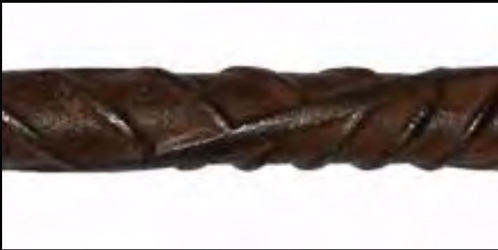
Twisted deformed CW.60, 1963 (Grade 410)
