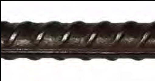
Hot-rolled deformed (D500N) 2017
