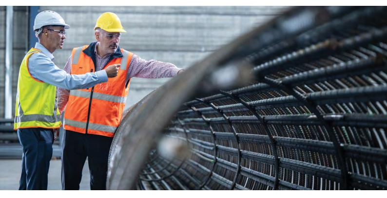
Over 140,000 tonnes of steel reinforcement is supplied in our market each year from unknown origins. If 'uncertified' steel is supplied on one of your projects then there is a high risk the reinforced concrete element may not perform. Even though design drawings might specify AS/NZS 4671 Steel for the reinforcement of concrete, it's difficult to prove conformance once the steel is fixed and the concrete is placed.
