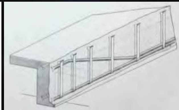
Hennebique System - Fishtail ends for anchorage
