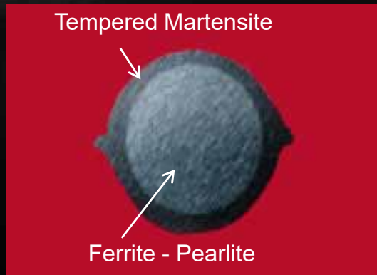
Quenched and self-tempered bar from 1983
