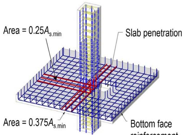
Top level reinforcement not shown for clarity
