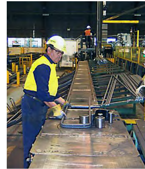
FIGURE 4 Factory Bending around Pins of Specified Diameters
