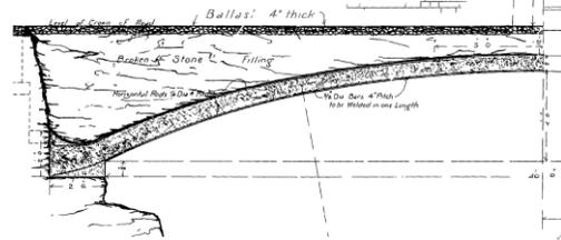
**Figure 4. Structural details of Monier arch bridge at Hilltop, 1899**
