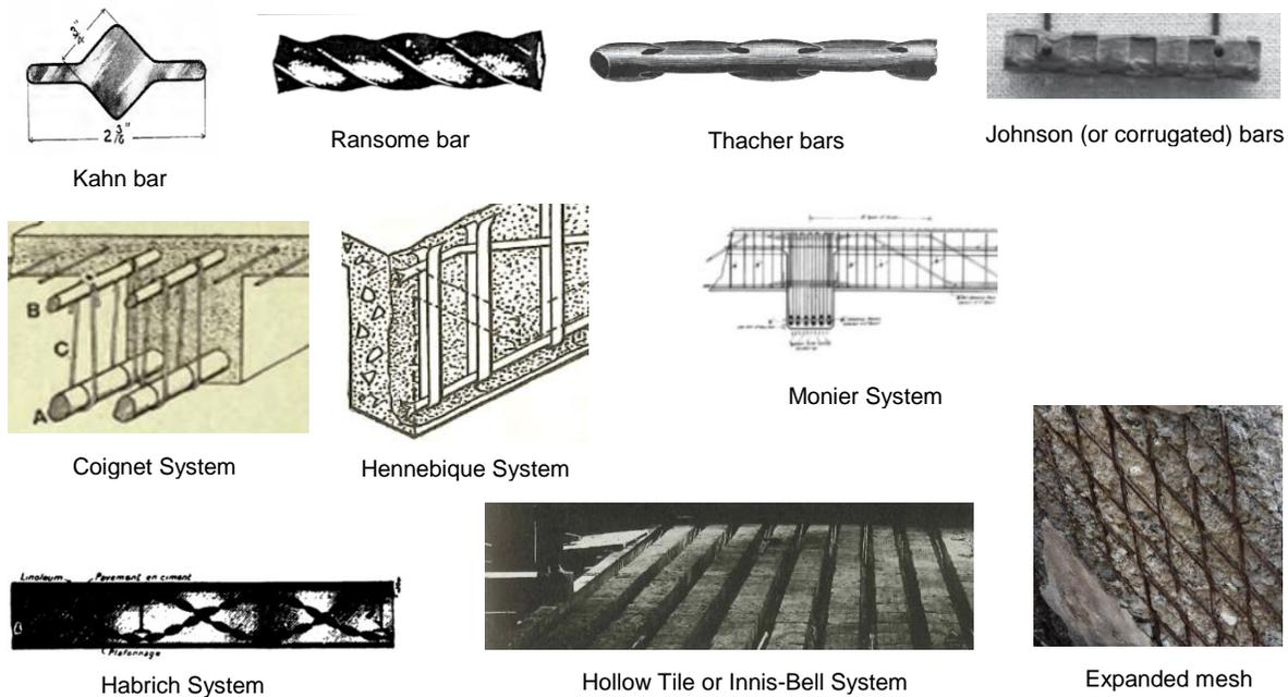
**Figure 1. Examples of patented steel reinforcement systems**
