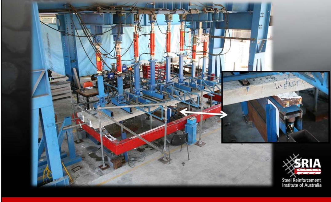
This shows a typical test set-up of one of the unrestrained DSOW slabs with its ends supported on the rollers, and with four line loads per span to simulate uniformly-distributed design loading.
