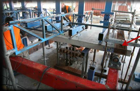
Simply-supported end tied down during initial lift at centre support, before hydraulic jacks above slab engaged
