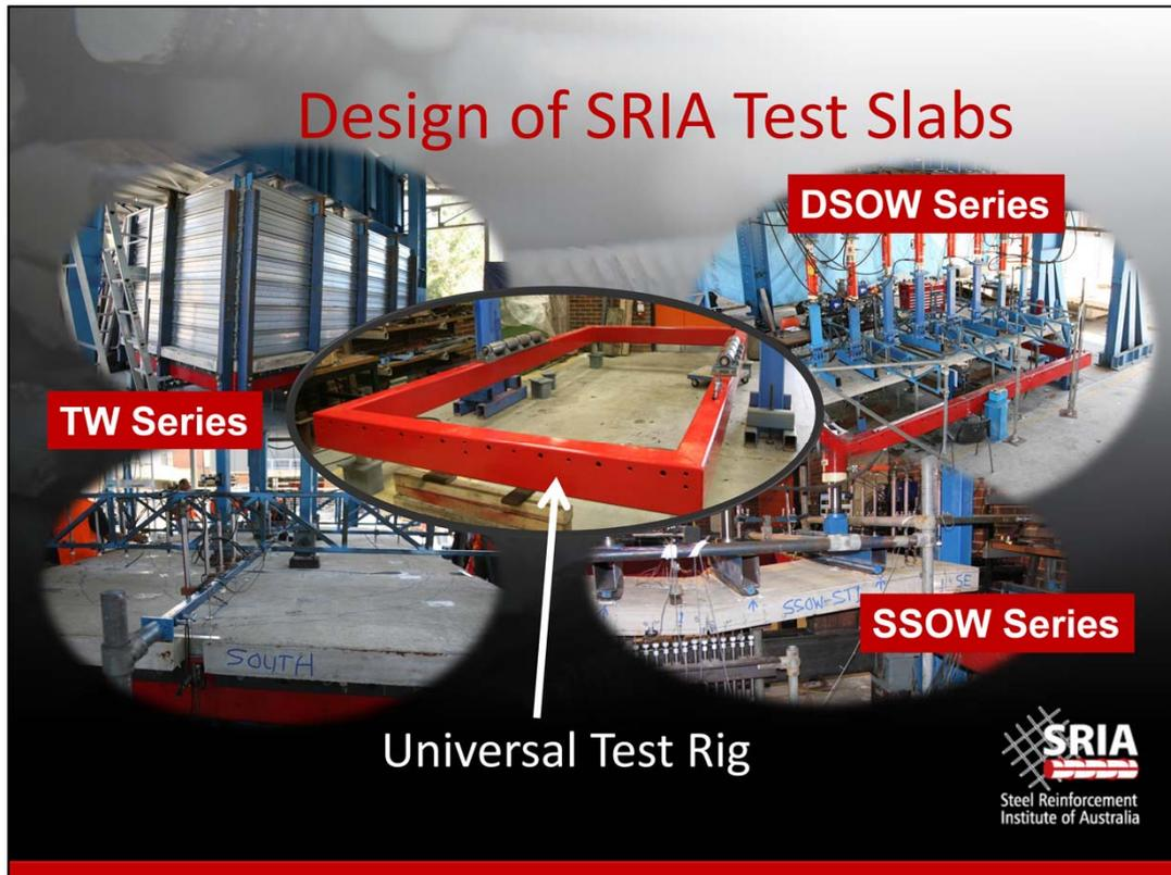
A universal test rig was designed to be used multiple times when testing three series of slabs: SSOW – Single-Span One-Way; DSOW – Double-Span One-Way; and TW – Two Way. All the slabs were nominally 110 mm deep.
