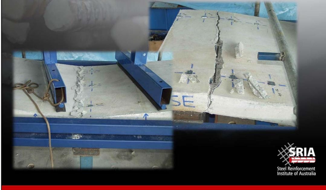
These photographs show the slab after the applied load was fully released. The main tensile bars had broken in the positive and negative hinge regions. This confirmed that the edge restraint detail was suitable for the main test series.
