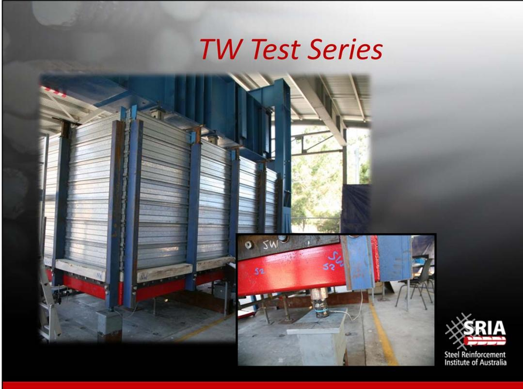
The test set-up involved loading the slab with water, with the temporary steel tank walls evident here. The small inset photograph shows one of the load cells used to record the vertical reactions during testing.
