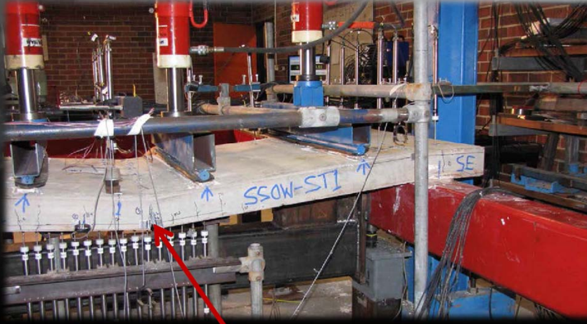
Fractured Bottom SL92 Bars
