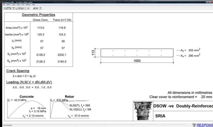
Using the best available estimates for the geometric and material properties of the test slabs, moment-curvature analysis was used to study the behaviour of the doubly-reinforced Class L cross-sections in negative or positive bending. This slide shows a summary-input screen of the software used.
