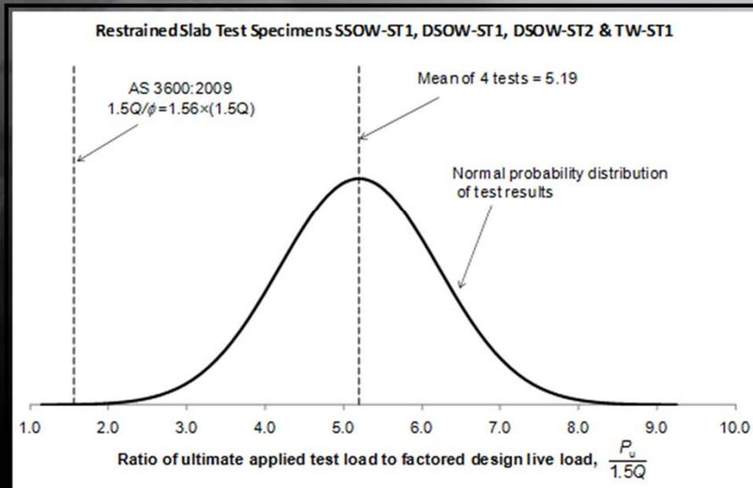
For slab SSOW-ST1, load ratio  $P_u/1.5Q$  was a very large value of 5.32. For slabs DSOW-ST1 and DSOW-ST2, it was 4.25 and 4.13, respectively, even with support settlement. For TW-ST1 it was 6.52 or 5.75 with the slab modelled as two one-way strips or as two-way, respectively. The mean value was 5.19, which is 233% above a value of 1.56 corresponding to collapse by flexural failure in design.
