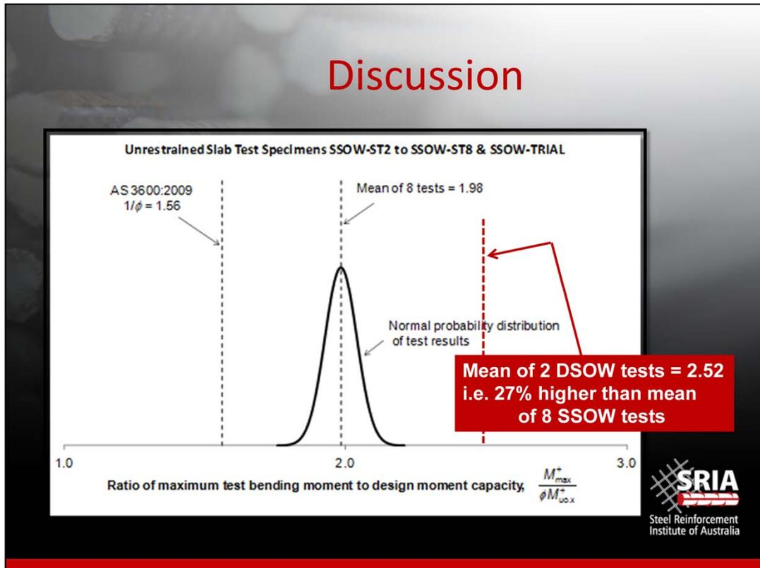
The values of moment ratio for DSOW-ST3 and ST4 were both about 2.52, which is significantly higher (about 27%) than the mean of 1.98 for the eight unrestrained SSOW slabs shown again here. A detailed investigation was made to explain this apparent anomaly.
