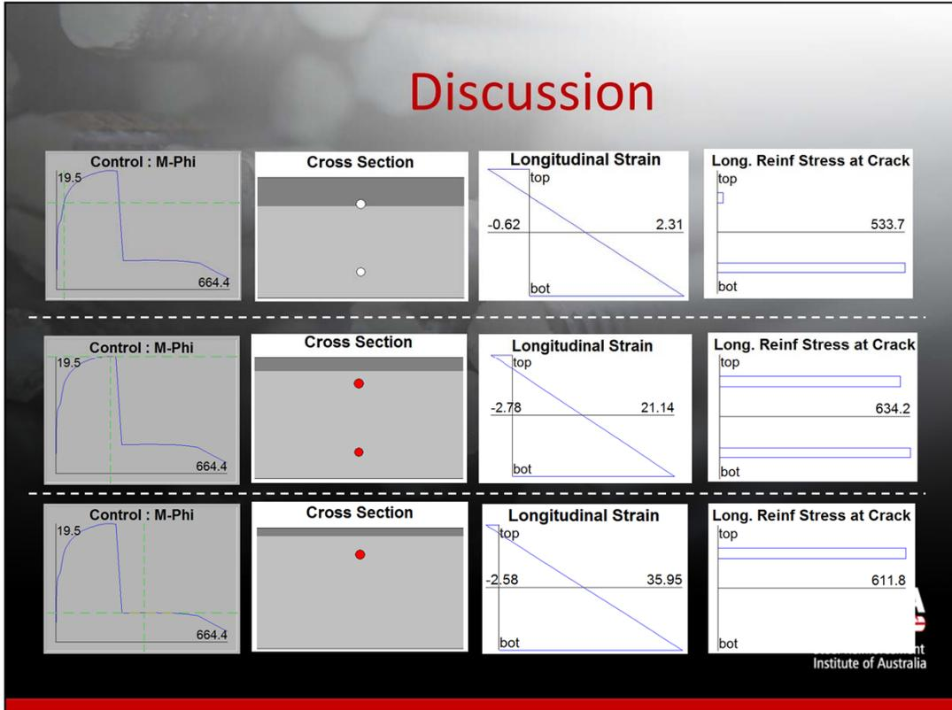
Here the results of the moment-curvature analysis are shown at three different curvatures.
