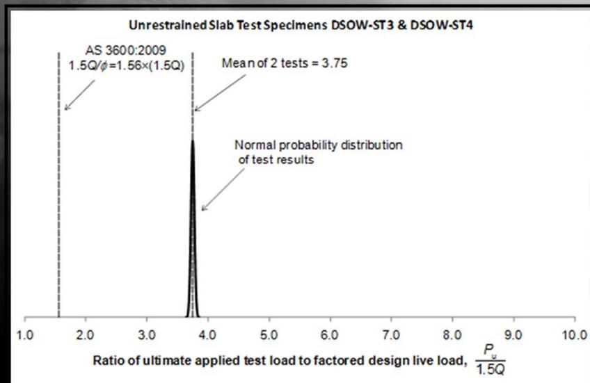
For slabs DSOW-ST3 and DSOW-ST4 (the latter initially subjected to support settlement) similarly high values of the load ratio of 3.77 and 3.73 occurred. The mean value of 3.75 is 140% above 1.56 corresponding to collapse by flexural failure in design.
