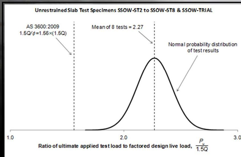
For slabs SSOW-ST2 to ST8 & SSOW-TRIAL supported on rollers, the values of load ratio  $P_u/1.5Q$  varied from 2.11 to 2.54, with a mean value of 2.27 which is 46% above a value of  $(1/\phi) = (1/0.64) = 1.56$  corresponding to collapse occurring for design in accordance with AS 3600– 2009.
