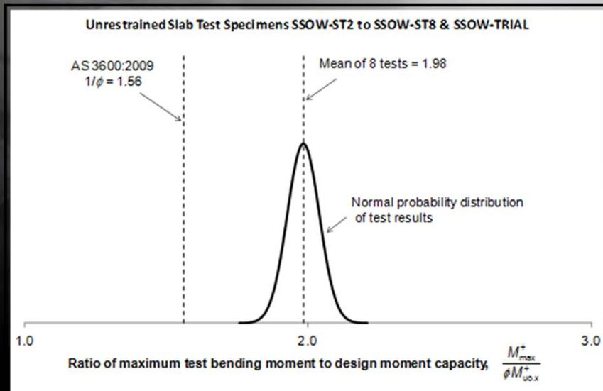
For the same SOW slabs, the values of moment ratio varied from 1.93 to 2.08, with a mean of 1.98 which is 27% above a value of 1.56 corresponding to flexural failure.
