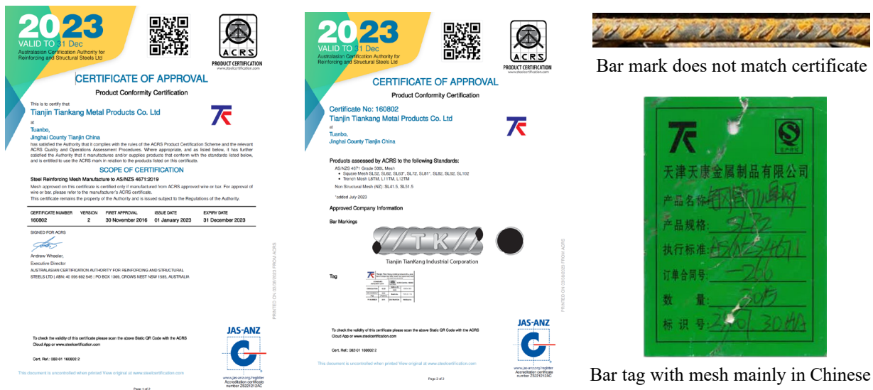
Figure 3 Bar mark on product does not match bar mark on 2023 ACRS certificate and bar tag difficult to interpret and not compliant
