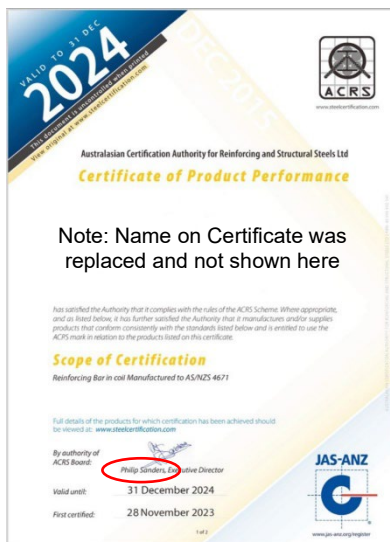
Figure 2 Fraudulent (older style) compliance certificate with date and company details altered
