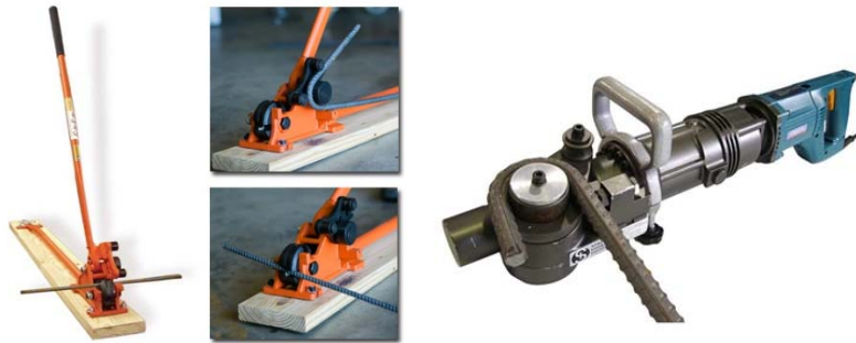
Figure 12. Examples of manual (left) and electric (right) bending tools.
