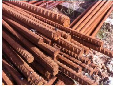
Figure 9. Example of acceptable surface corrosion.
